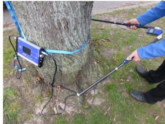
Using Triangulation method and electronic calipers to measure positions of all MP
