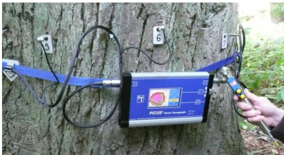
Using Triangulation method and electronic calipers to measure positions of all MP
